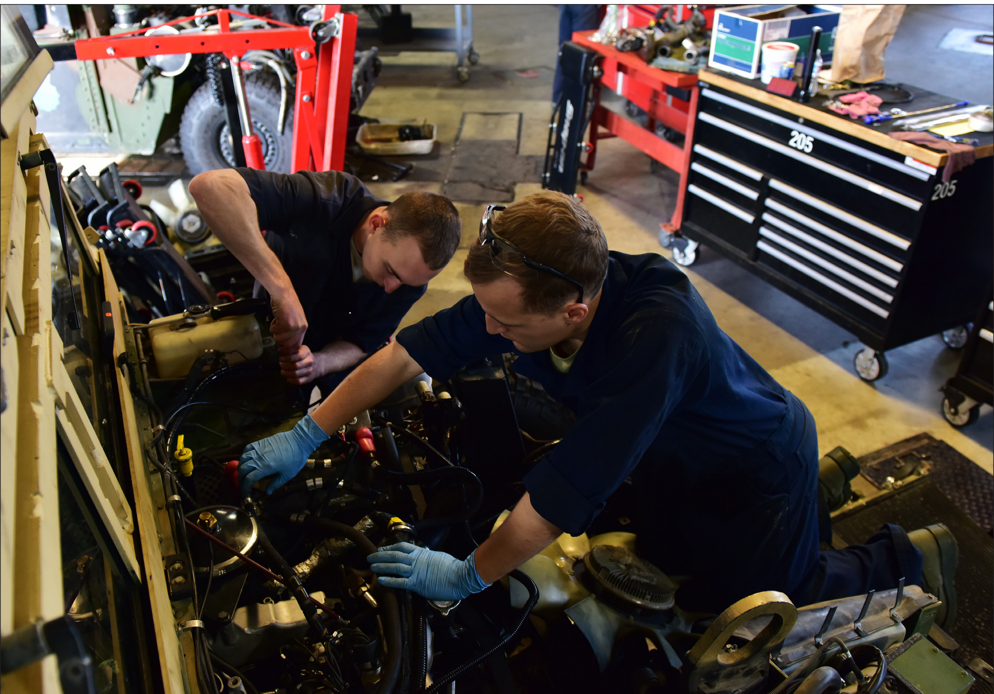
Senior Airman Cody Smith, right, and Airman 1st Class Benjamin Deeren, both vehicle maintenance journeyman assigned to the 509th Logistics Readiness Squadron, tighten engine attachments of a Humvee at Whiteman Air Force Base, Mo., Nov. 2, 2016. Loose connections can lead to more damages to the engine or cause it not start at all.
